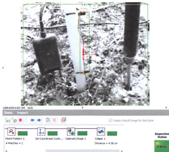
Fig. 8: Measurement result of asparagus stems
